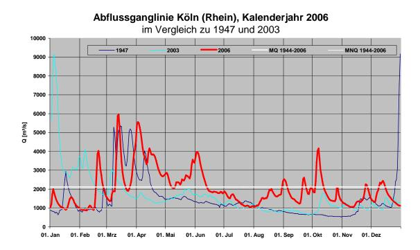
It can be seen that several times between the middle of January and the middle of February discharges fell below the long-term mean low-flow discharge (MNQ). This period of less discharge was, however, superseded as from 18 February by above-average water levels of long duration. The crest of the flood wave on 13 March 2006 was, however, at  $5,950 \text{ m}^3/\text{s}$  not unusually high – floods of such magnitudes are expected in Cologne about every one to two years.
