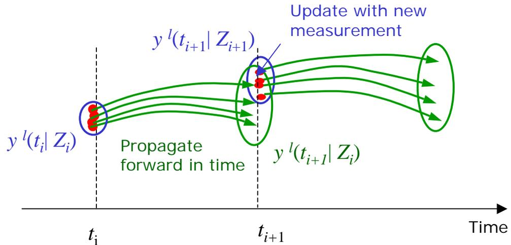
Ensemble filtering propagates only replicates (no PDFs).
